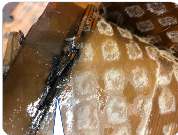
Primary winding (circled): Design is outer secondary / primary / inner / secondary (Primary has 1600 Windings with approximately 80 windings/layer – Secondary has 16 layers each (one sheet per layer)
